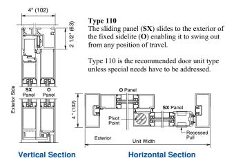
7'-0" to 9'-0" Upto 16-0" (4877) (2134 - 2743) $\langle\!\!\!\langle$ 7'-2 1/2" (2197) Optional M<u>untinBar</u> 413/4 (1060)(O-SX Reverse) Type O-SX-SX-O Max. SlideOpng. Max. SlideOpng.  $\Rightarrow$  $\ll$ Emergency Exterior
